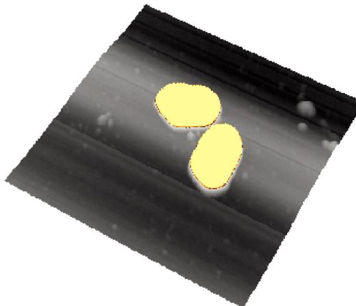
Figure 1: AFM image of  $\alpha$ -Fe<sub>2</sub>O<sub>3</sub> particles prepared by wet way, section in *xy* plane (scan size: 680 × 680 nm)
