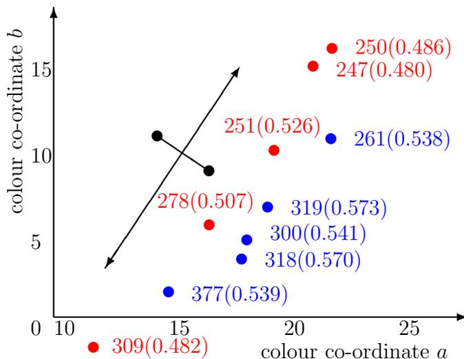
Figure 2: The colour co-ordinates of  $\alpha$ -Fe<sub>2</sub>O<sub>3</sub> samples and directions of influence of mean diameter (arrow) and asymmetry parameter (line with disks)
